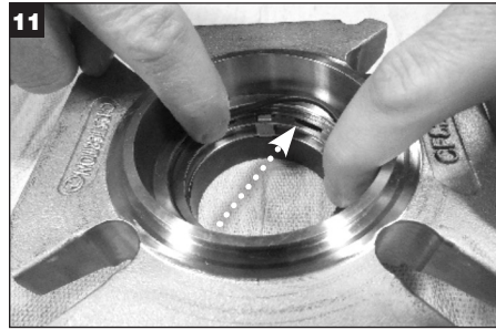
Carefully invert the gland and place it on a clean cloth to protect the inboard seal ring surface. Apply a thin film of grease to the remaining Stationary O-ring (X) and install it in the inside diameter groove in the gland.
