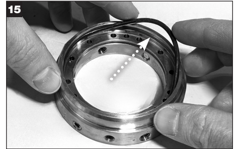
Apply a thin film of grease to the Lock Ring Holder O-ring (U) and insert it into the larger inside diameter lock ring groove.
