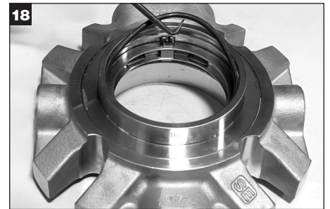
18 Remove the inboard Stationary O-ring (X) from the adapter and discard.
