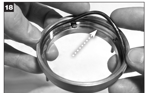
Apply a thin film of grease to the outboard Rotary O-ring (W) and insert it into the inside diameter holder assembly groove.
