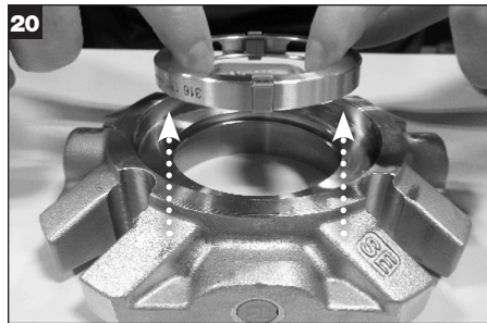
20 Remove the drive channel from the gland; remove the channel clips and the flow deflector from the drive channel and discard.
