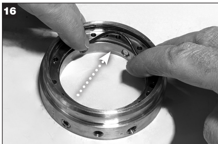
Apply a thin film of grease to the Lock Ring Sleeve O-ring (Y) and insert it into the smaller inside diameter lock ring groove.
