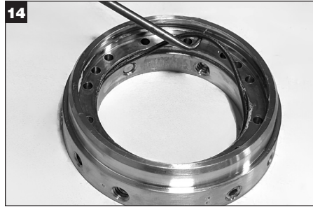
14 Remove the Lock Ring Sleeve O-ring (Y) and discard.
